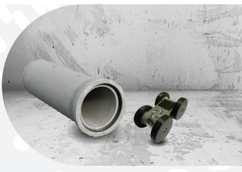
The NuROLL robot has been designed to inspect areas with access constraints and/or in environments where radio transmissions are normally restricted. Its modularity allows it to be used in several fields (nuclear, hydraulic/water and sanitation, etc.) thanks to the possibility to incorporate various features such as cameras or measurement sensors. Wireless, it can be The NuROLL is a wireless device controlled with a joystick.
