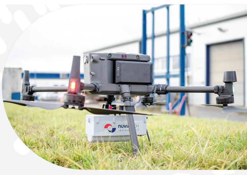
The DRONES-G MINI module with integrated radiation detector is a compact and lightweight system to be used with small commercially available drones, while maintaining sufficient detection sensitivity for measurements in the event of a radiation accident or for routine monitoring by security forces. The system was developed in cooperation with the State Institute of Radiation Protection in Czech Republic as part of their Security Research Program.
