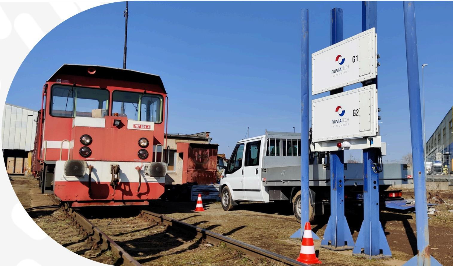
The detection gate is equipped with two 25 l scintillation detectors, designed for quick and easy inspection of cars and trucks transporting scrap metal. The high sensitivity of the detection system guarantees high reliability of detection of potential sources of ionizing radiation.
