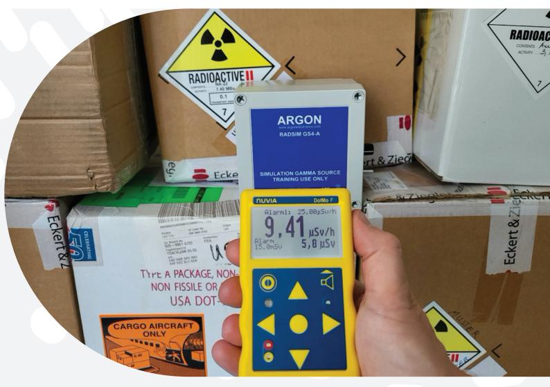
The new training devices DolMo SIM (dose and dose rate meter) and CoMo-170 SIM (contamination detection device) are designed for the practiceoriented training of radiation protection officers and first responders. The technically modified devices respond to radio waves (DolMo SIM) or to magnetic fields (CoMo SIM) and can therefore be used for training scenarios even without radioactive sources.
