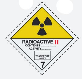
Example: Hazard labels for radioactive substances
