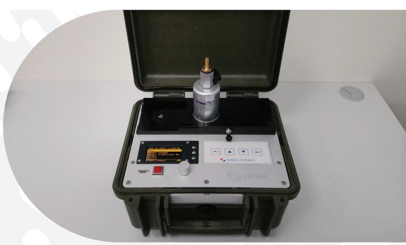
The NuRADON SOIL system intended for in-situ measurement and evaluation of radon concentration in soil by Lucas chambers. The system undertakes data processing and determination of radon volume activity, and is compatible with different volumes of Lucas chambers. It has been designed for the determination of the radon index of land, as such can operate with a large number of measurement chambers. The system is very easy to operate without any pre-requisites.
