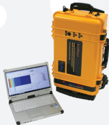
Portable version with a smaller detector volume (4" x 4" x 8"). Neutron detector not included, sold separately.
