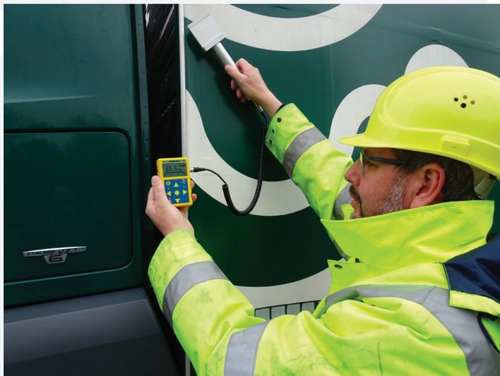
**NuSEARCH Kit** - A choice of detectors designed to easily search for the contaminated material and provide essential information to the nuclear authorities. The combination of the easy-to-use handheld device DoMo and a highly sensitive probe allows the user to **confirm the presence of radioactivity and trigger the adequate response.**
