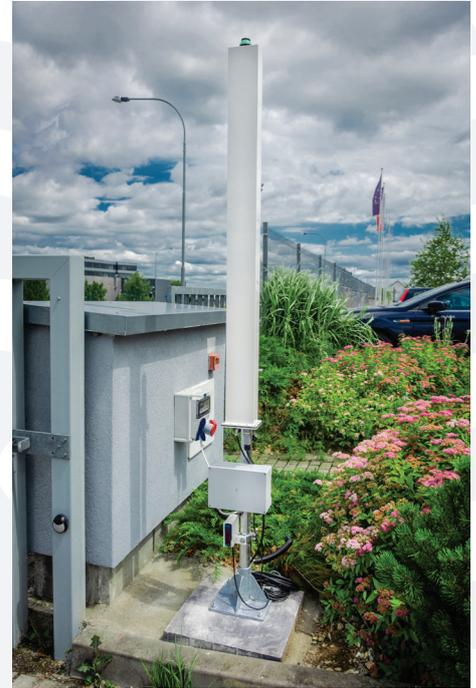
**NuCLEARANCE Lite** - cost effective portal monitoring system providing essential monitoring to detect radioactive material accidentally hidden in the scrap metal.
