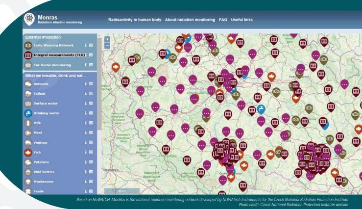
NuWATCH is a comprehensive early warning network for radiation monitoring and analysis based on a multiple sensors distributed over a medium to large area. This network of detectors connected to the RADIS software can display a near real-time map of the radiological conditions.
