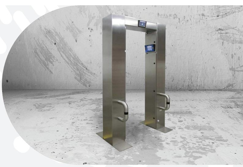
Working with radioactive materials carries the risk of contaminations. A check point for radioactivity enhances the safety of humans and the environment. Large area plastic scintillation detectors in the pillars of the Portal-S measure ionising radiation. Light barriers and an automatic analysis guarantee an easy and fast control.
