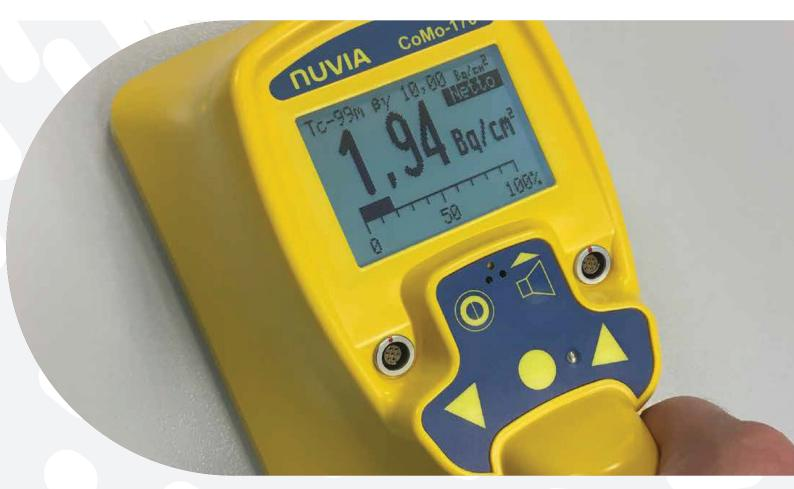
Working with open unsealed radioactive material can lead to contamination of persons and surfaces. Therefore, persons and equipment leaving control areas have to be checked. Mobile contamination monitors such as the CoMo-170 or CoMo-300 are used for direct and indirect contamination measurements. Combined with dedicated accessories, these powerful measuring devices provide a complete solution for contamination control and clearance measurements.
