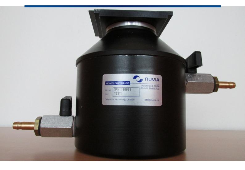
LUCAS is a complete detection system designed for radon volume activity measurement in air, soil and water samples.
