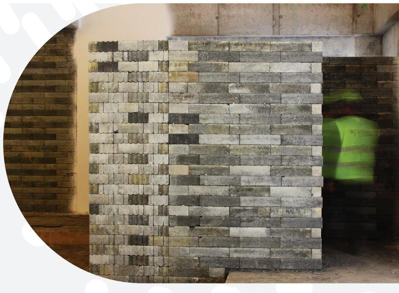
NuRAD 8200 is a special modular shielding material made of lowbackground and high-density concrete in unified segments, modules and related building components with unique features designed for the nuclear industry, safety and laboratory application.
