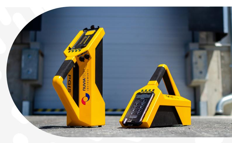
The instrument is designed for portable or backpack application of radiation detection and monitoring in a variety of environments. The system is auto calibrated by natural photo peaks, consisting of a detector unit, integrated with GPS, and a data logger unit based on Android portable devices, such as a smart-phone, a tablet or a notebook. The detector is equipped with a NaI(TI) crystal with a volume of 0.347 liters.
