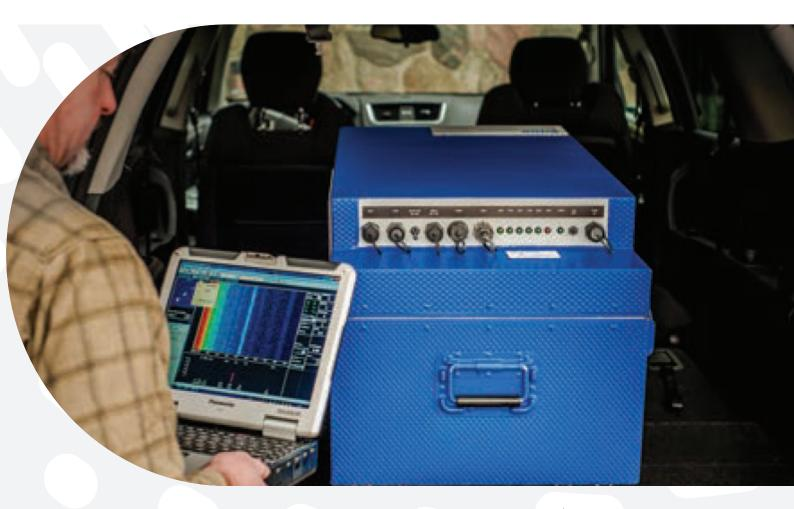
SIRIS is a Stand-off Integrated Radiation Information System based on PEI's expertise in radiation measurements on moving platforms. Proprietary algorithms provide immediate Radiation detection, directional radiation recognition, isotopes identification (RIID), real-time activity calculation of natural and man-made isotopes, customizable notifications and crew safety alarms. The SIRIS – is a newly developed system for CBRNe and Homeland
