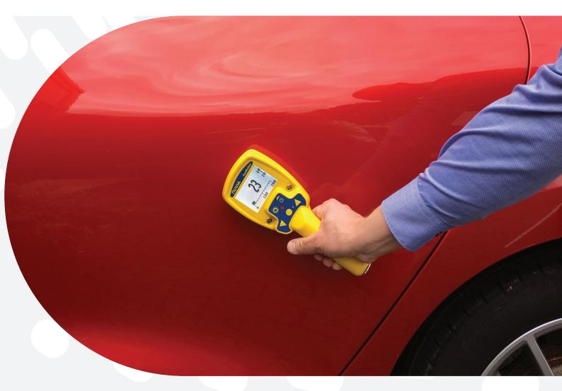
An essential part of international customs is prevention of smuggling, especially drugs, weapons, explosives and cigarettes. RadReflex 2, NUVIATech Instruments contraband detector is a fast and secure way to check cavities within vehicles. Using reflected radiation from a small radioactive source is possible to identify areas which have been modified for smuggling.
