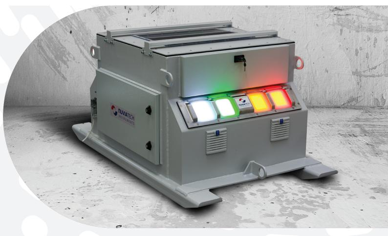
GEM is a rapid bulk monitoring system for radiological characterisation of soil, concrete, bricks or other material. The system is capable of a real-time assay to determine the activity level within the excavator bucket. Each bucket typically requires just 10 seconds to complete a measurement depending on isotopes and required detection limits. Once completed, a light on the system automatically turns on to indicate the level of contamination and therefore its waste category.
