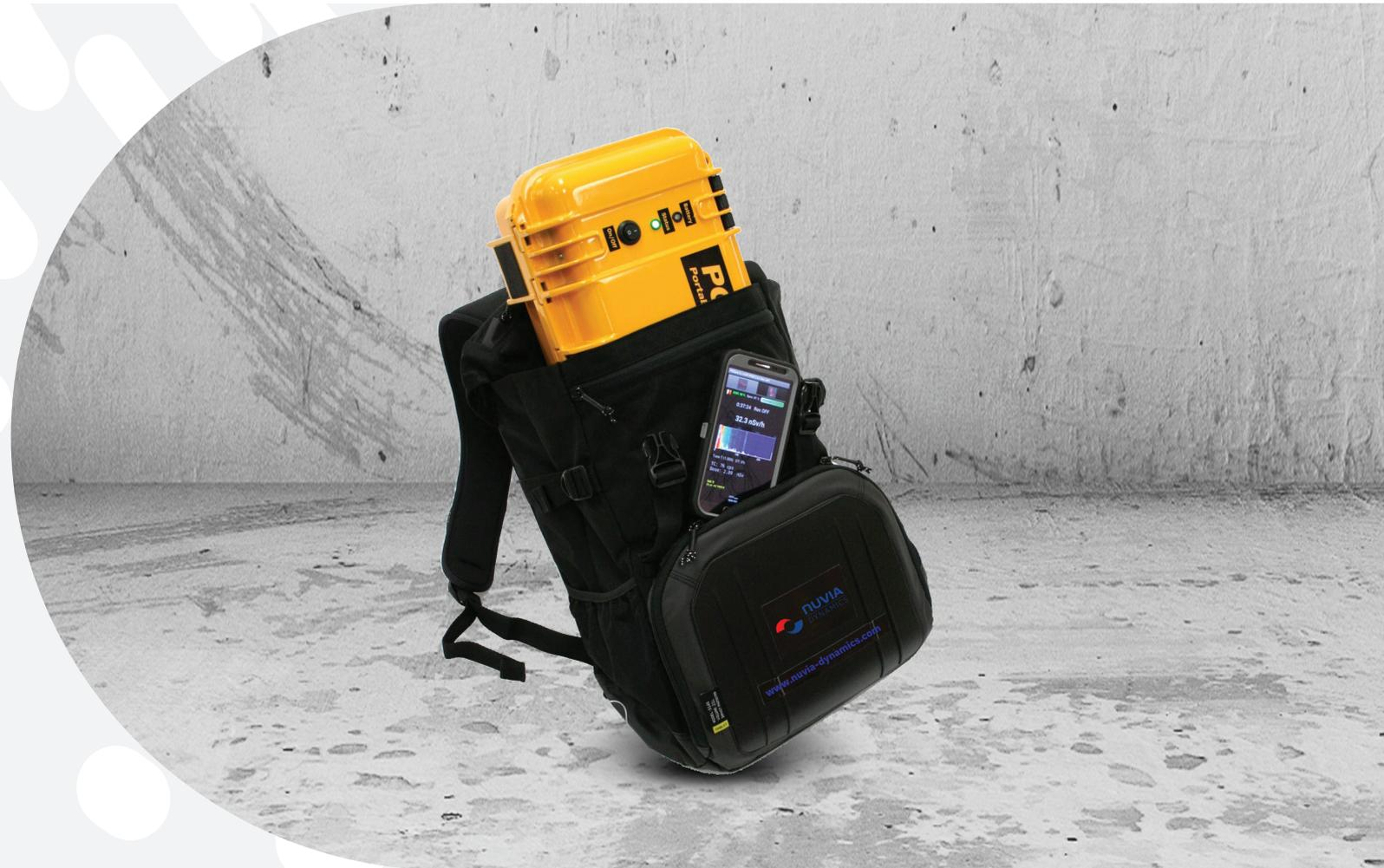
The instrument is designed for portable or backpack application of radiation detection and monitoring in a variety of environments. The system is auto calibrated by natural photo peaks, consisting of a detector unit, integrated with GPS, and a data logger unit based on Android portable devices, such as a smart-phone, a tablet or a notebook. The detector can be equipped with a NaI(Tl) crystal of various volumes ranging from 0.347 liter up to 2 liters.
