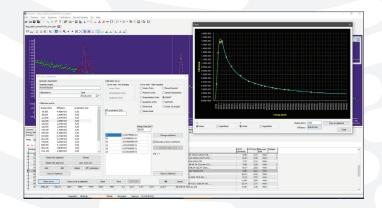
**MDA/MSA determination:** The module contains routines to determine the minimum detectable (significant) activity using the Currie method and KTA. The results are shown in the form of a table and in a report.
