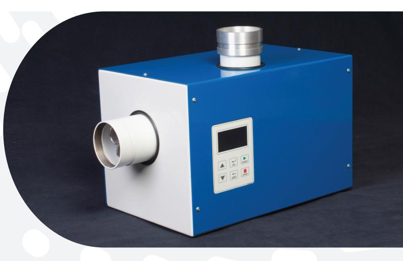
EGS is a high volume air sampling system used for capturing radioactive aerosols, emissions, dust and other air pollutants contained in sampled ambient air. Sampled air passes through removable filters that are subsequently analysed in a laboratory to evaluate volume activities of captured particles.
