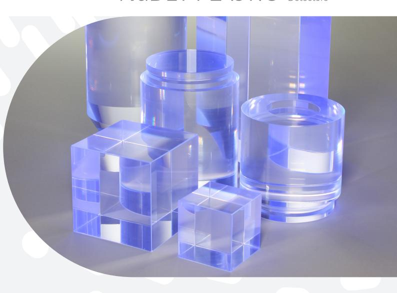
PLASTIC is a range of plastic scintillation detectors Plastic scintillators are solid solutions of luminophores in polymer characterised by a short decay time and a resistance against high dose rates. They are widely used in detection systems for their efficiency, high reliability and variety of shapes and sizes.
