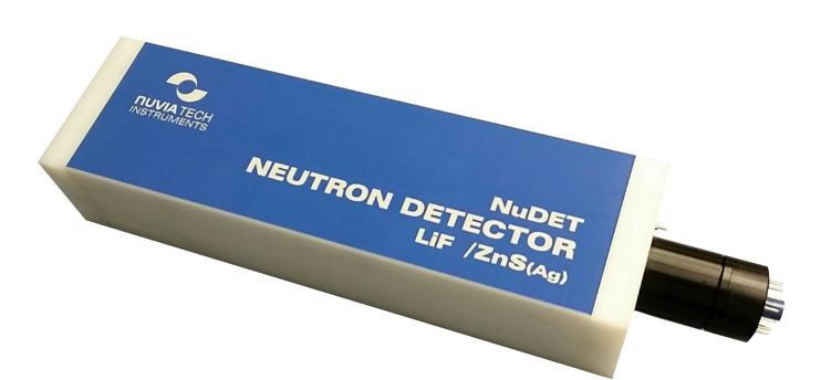
NEUTRON - innovative <sup>3</sup>He-free neutron detectors with high gamma rejection capability. The detection module is based on a plastic light guide coated with a <sup>6</sup>LiF/ZnS:Ag detection layer.
