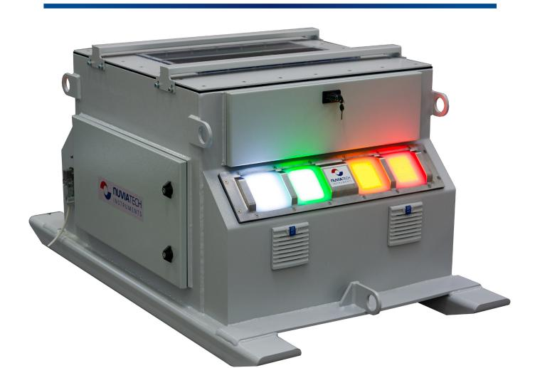
GEM is a rapid bulk monitoring system for radiological characterisation of soil, concrete, bricks or other material. The system is capable of a real-time assay to determine the activity level within the excavator bucket. Each bucket typically requires just 10 seconds to complete a measurement depending on isotopes and required detection limits. Once completed, a light on the system automatically turns on to indicate the level of contamination and therefore its waste category.
