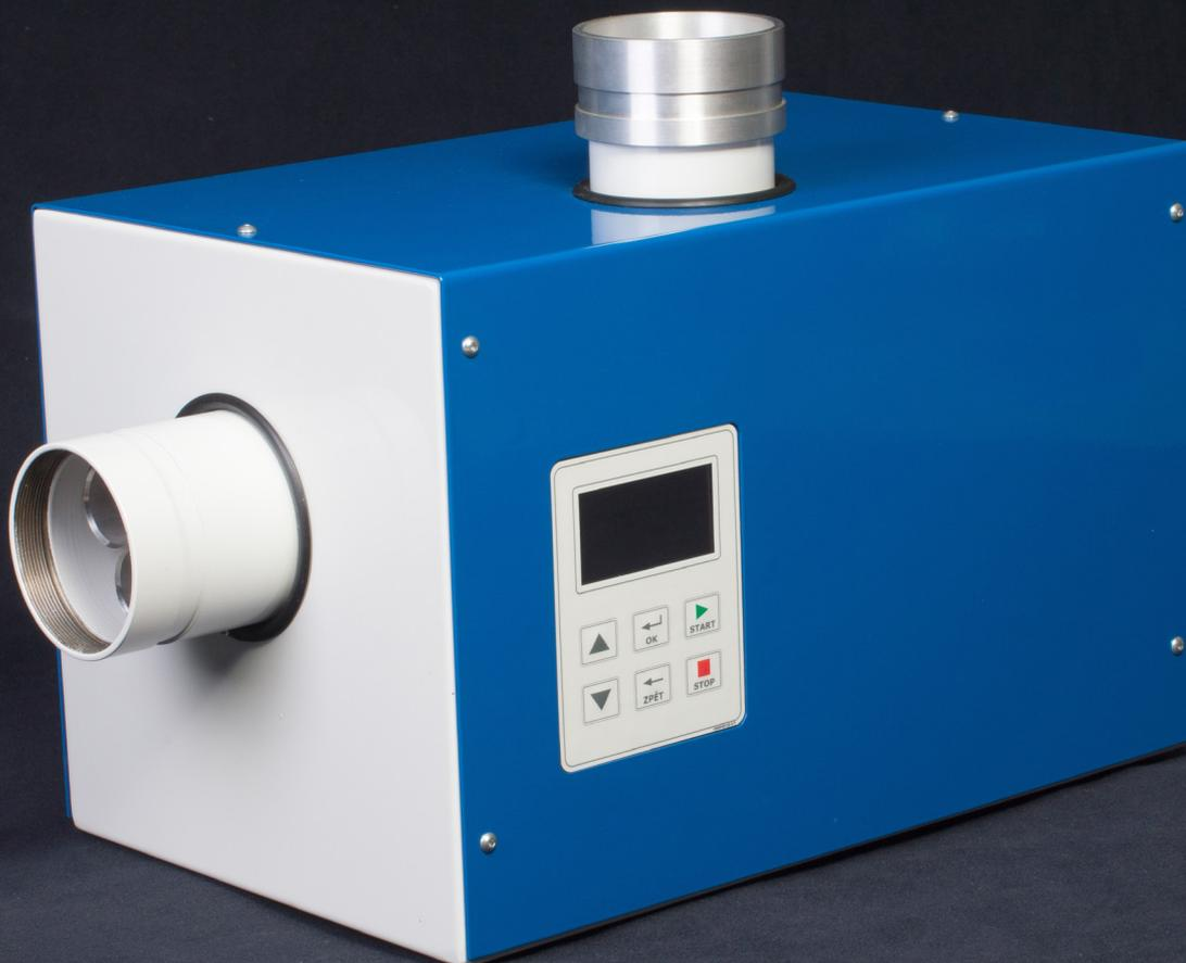
EGS is a high volume air sampling system used for capturing radioactive aerosols, emissions, dust and other air pollutants contained in sampled ambient air. Sampled air passes through removable filters that are subsequently analysed in a laboratory to evaluate volume activities of captured particles.
